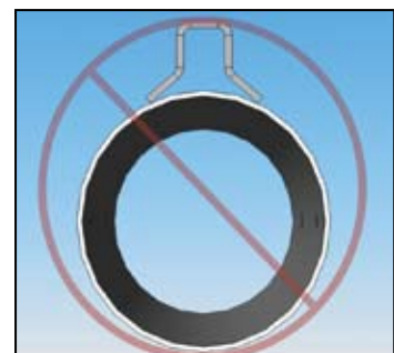
Figure 8: Incorrect hardware curvature
