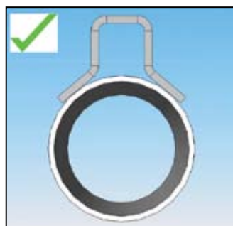
Figure 7: Correct hardware curvature
