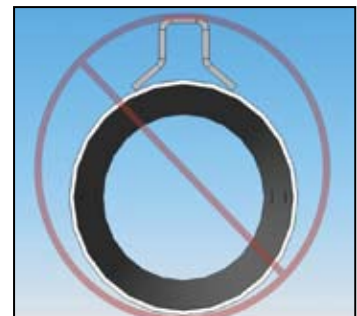
Figure 8: Incorrect hardware curvature
