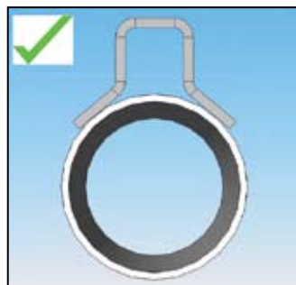
Figure 7: Correct hardware curvature
