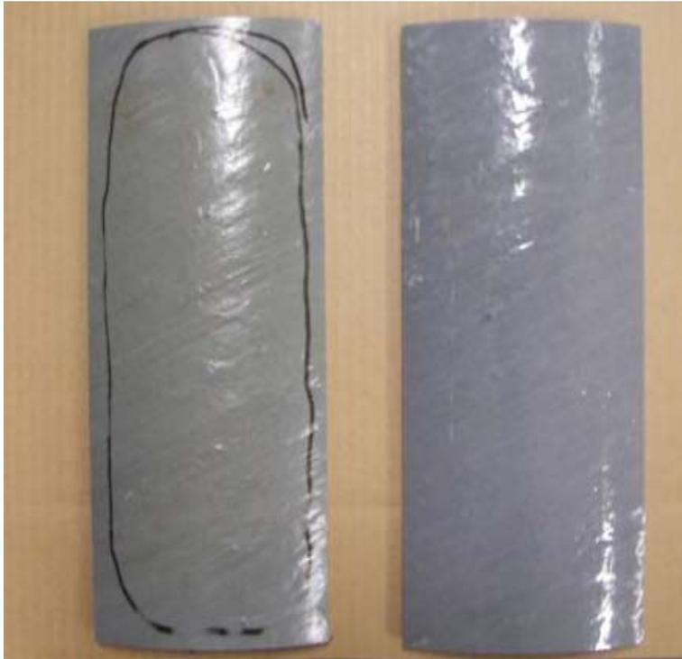
**Figure 1:** Weathering and UV Exposed Sample vs. Control Sample. (14,010h of QUV exposure on the left, with the unexposed control sample on the right). The one inch edge as shown on the exposed sample was removed prior to testing.
